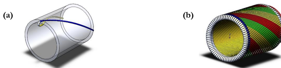
Fig. 1: Three-phase 4-pole alternator helical armature winding: a) one turn, b) full lay out of the winding.
